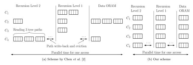
Figure 2: **Parallel runtime for a single OPRAM access.** The figure shows parallel runtime an OPRAM access performed for m = 4 clients and two Path ORAM recursion levels. For ease of exposition, only paths read by each client is shown.
