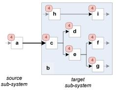
Figure 7: Conceptual view of functional model in which the external connection emanates from subsystem a and impacts parts of the target subsystem b.
